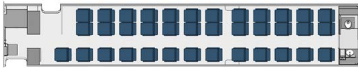
ERJ 135 INTERIOR CONFIGURATION 37 SEATS AT 31" PITCH
