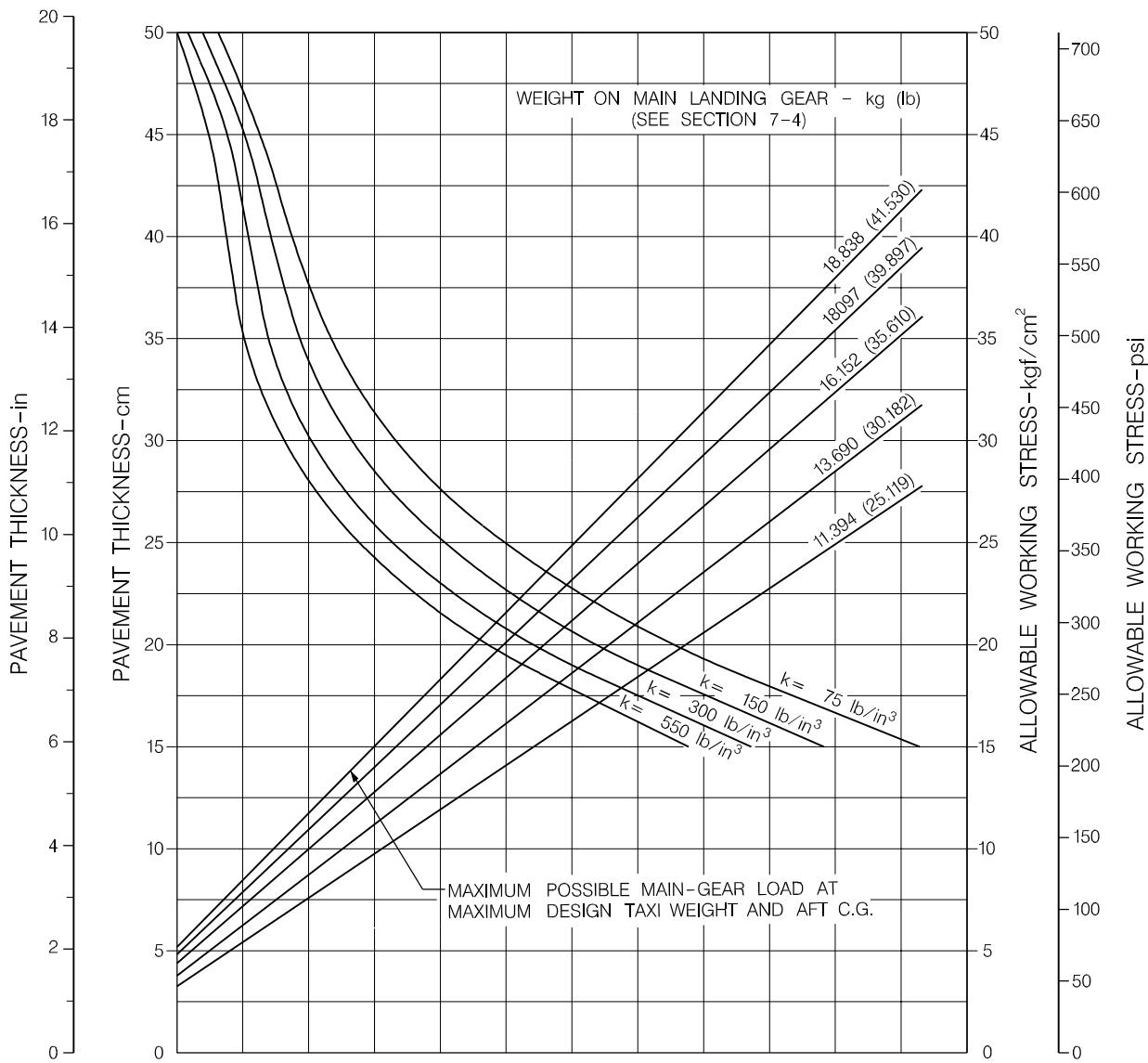
**NOTE:** THE VALUES OBTAINED BY USING THE MAXIMUM LOAD REFERENCE LINE AND ANY VALUE OF "K" ARE EXACT. FOR LOADS LESS THAN MAXIMUM, THE CURVES ARE EXACT FOR K=300 BUT DEVIATE SLIGHTLY FOR OTHER VALUES OF "K".
