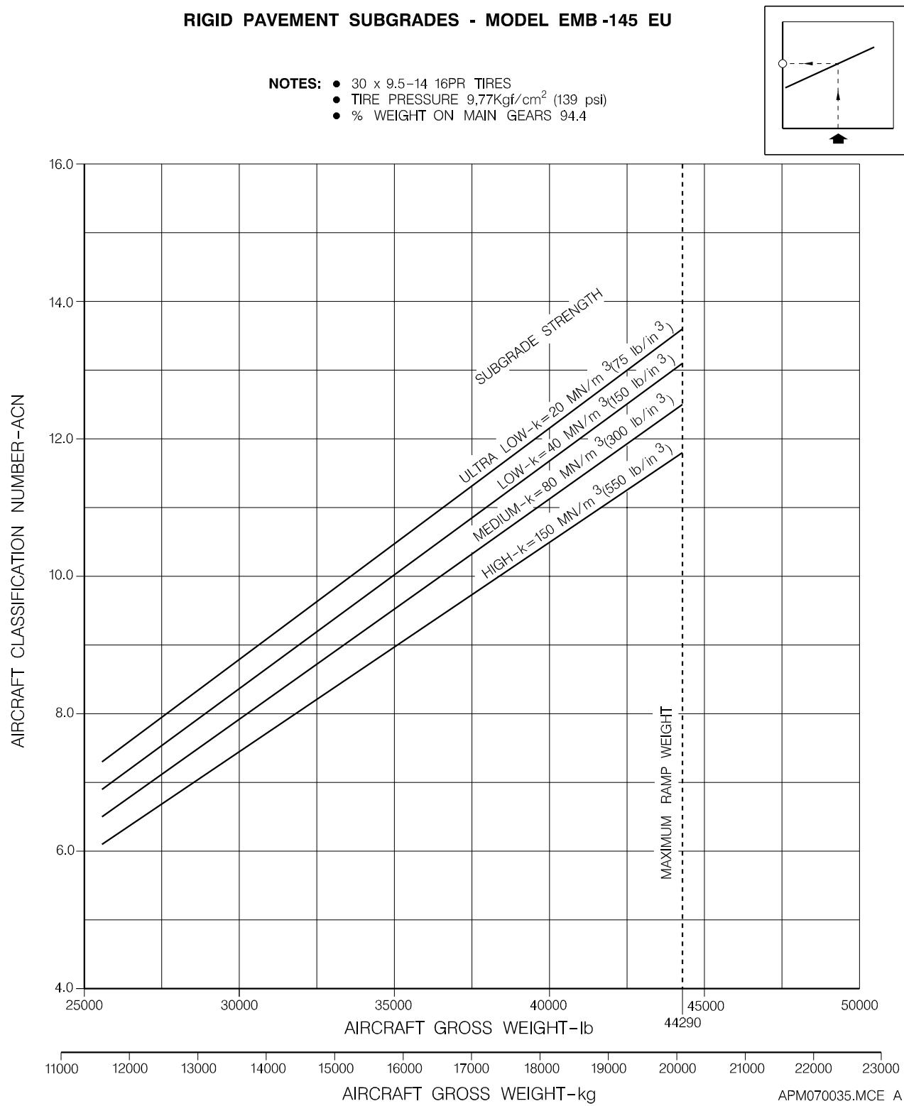
**Figure 7.9.2 - Aircraft Classification Number Rigid Pavement**
