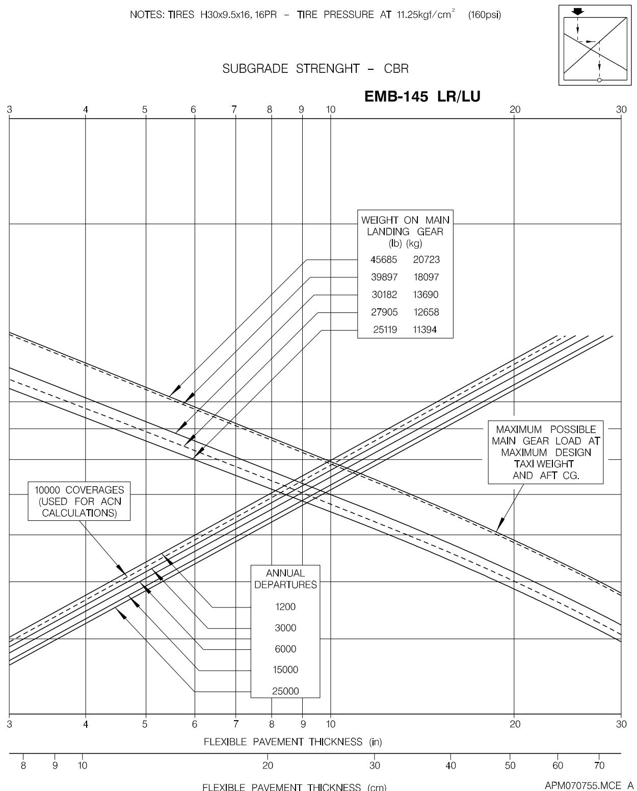
Figure 7.5.1 - Flexible Pavement Requirements - US Army Corps of Engineers Design Method
