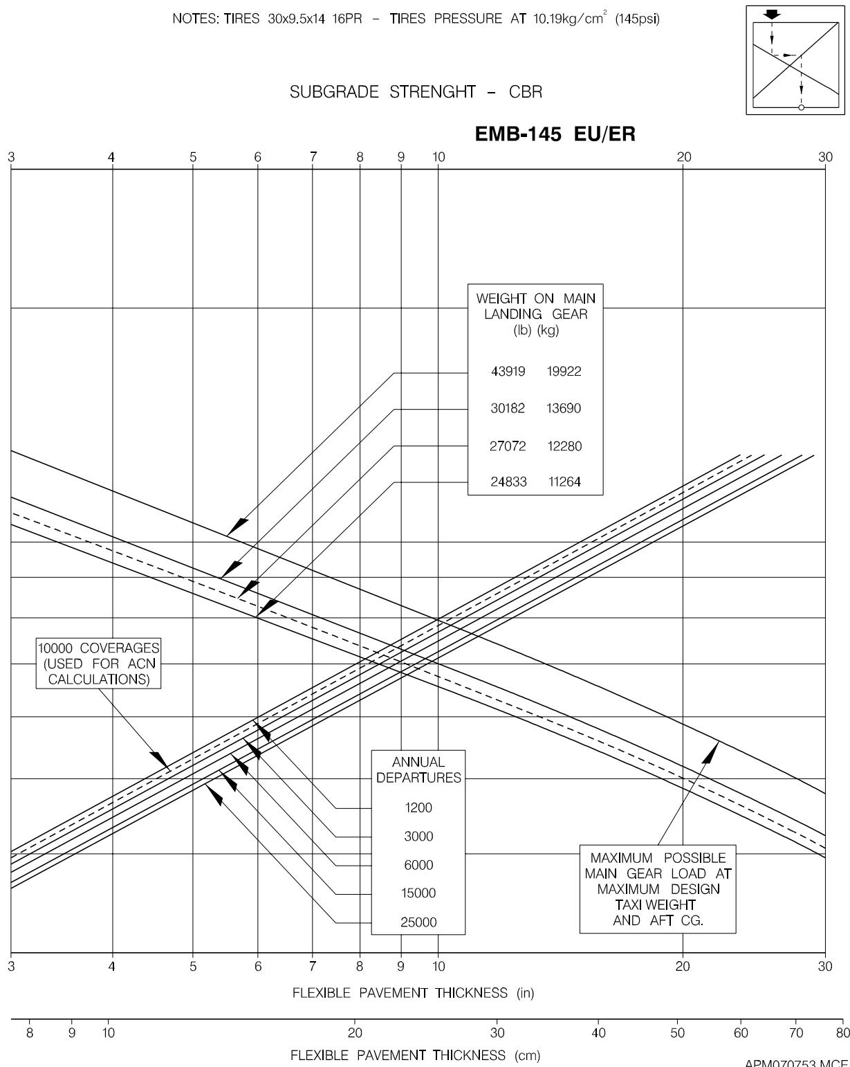
**Figure 7.5.1 - Flexible Pavement Requirements - US Army Corps of Engineers Design Method**
