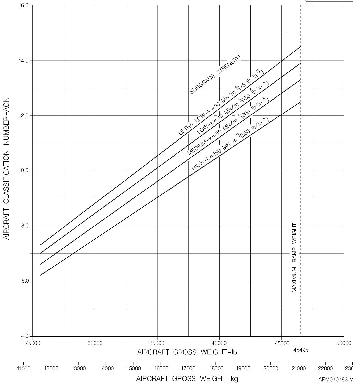
Figure 7.9.2 - Aircraft Classification Number Rigid Pavement
