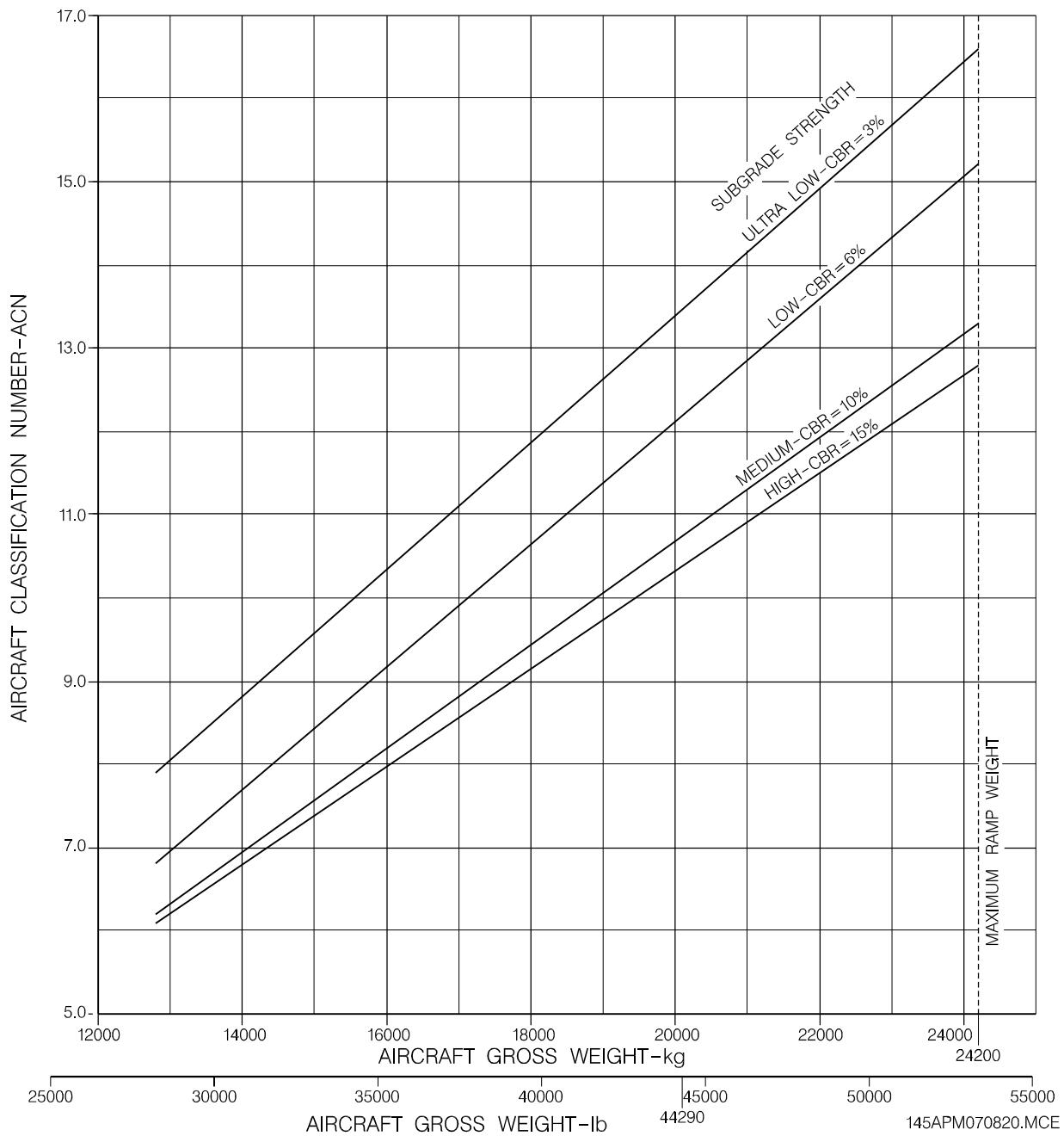
Figure 7.9.1 - Aircraft Classification Number Flexible Pavement
