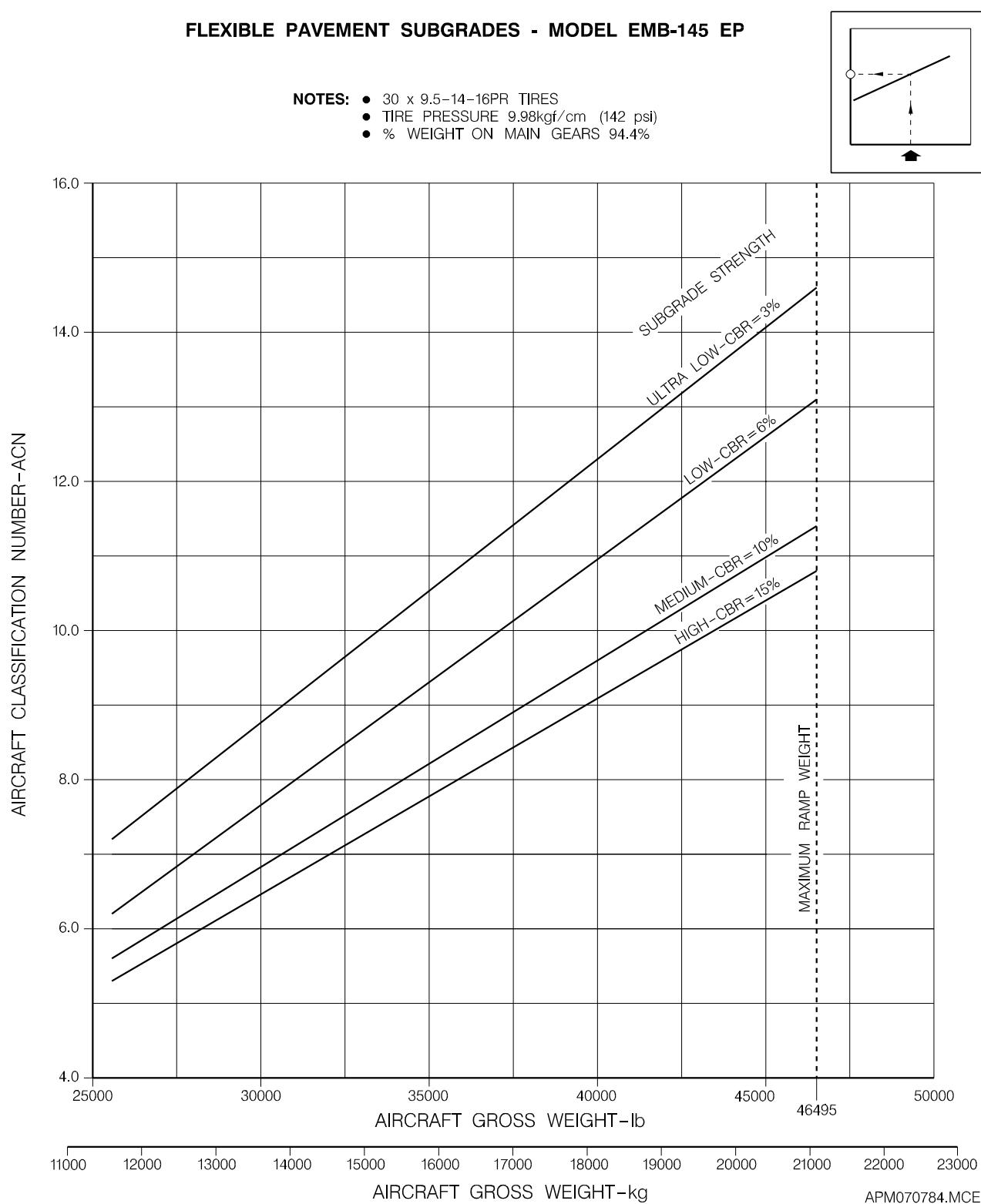
Figure 7.9.1 - Aircraft Classification Number Flexible Pavement
