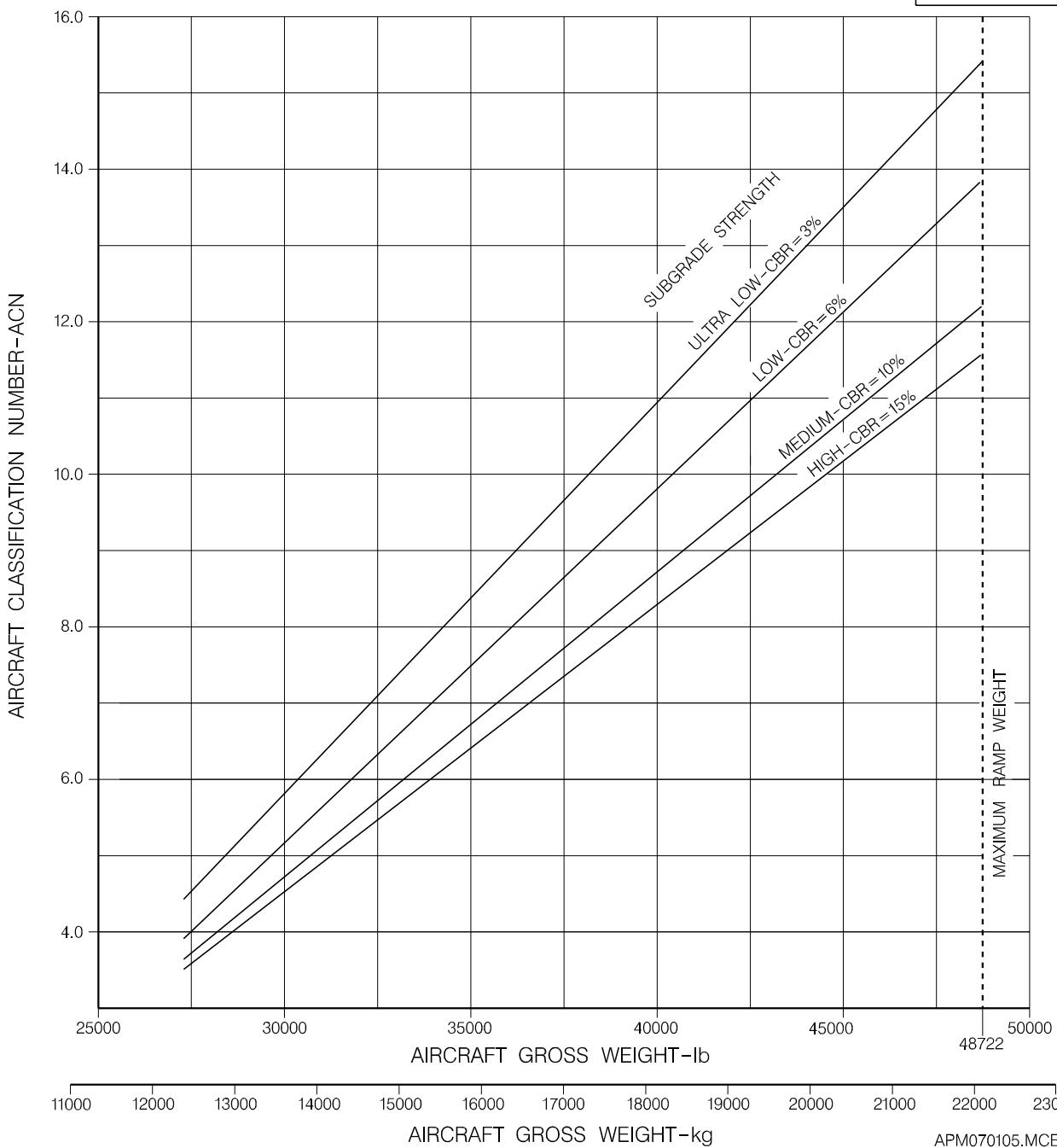
Figure 7.9.1 - Aircraft Classification Number Flexible Pavement
