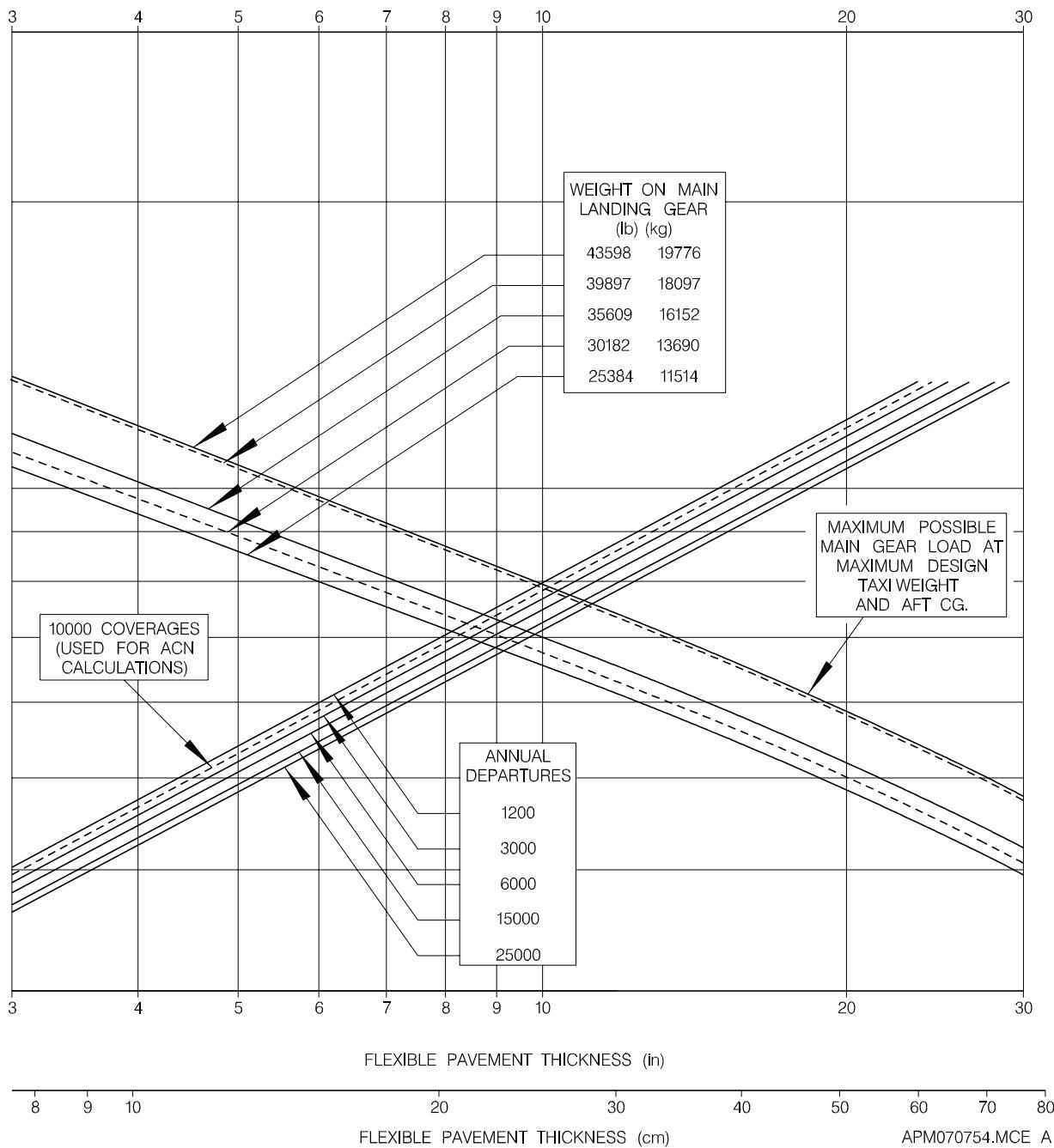
*Figure 7.5.1 - Flexible Pavement Requirements - US Army Corps of Engineers Design Method
