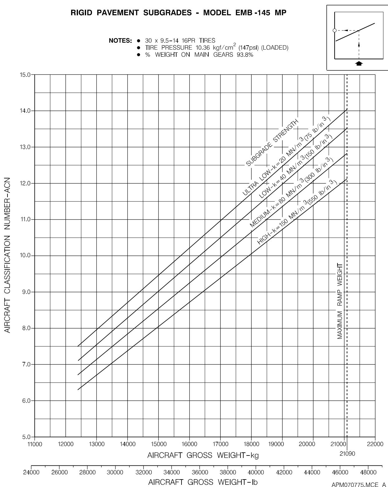
Figure 7.9.2 - Aircraft Classification Number Rigid Pavement
