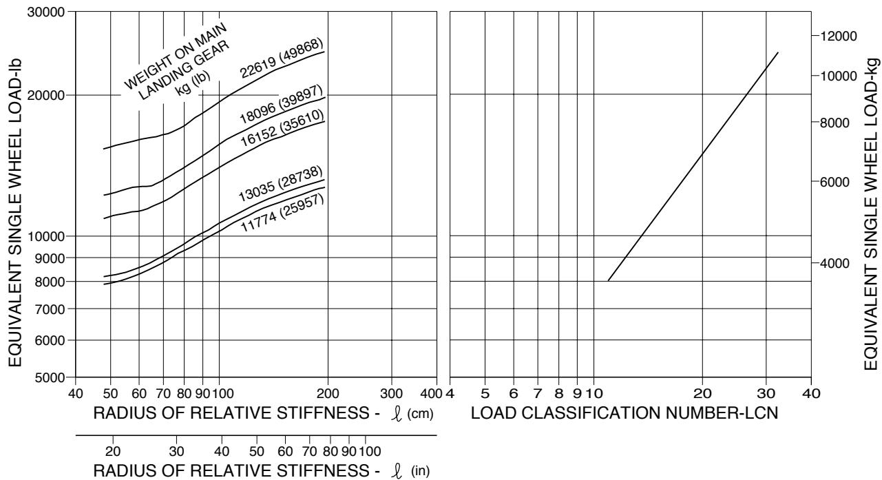
**NOTE:** EQUIVALENT SINGLE WHEEL LOADS ARE DERIVED BY METHODS SHOWN IN ICAO AERODROME MANUAL. PART 2, PAR. 4.1.3
