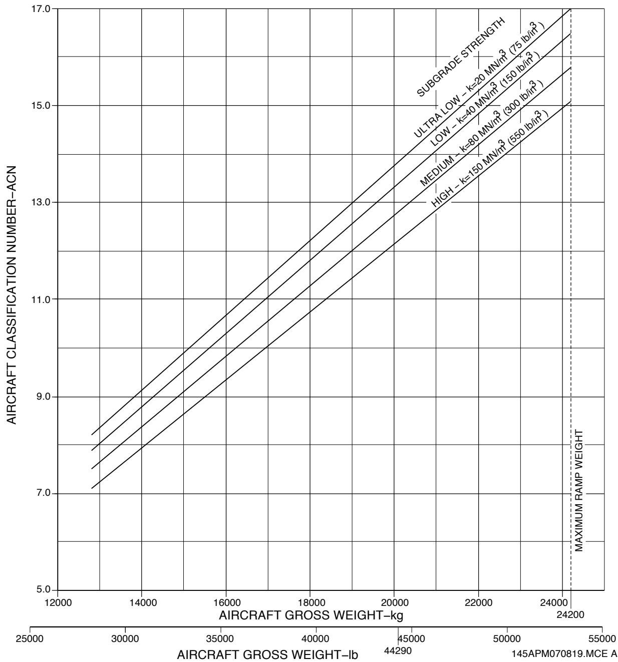
Figure 7.9.2 - Aircraft Classification Number Rigid Pavement
