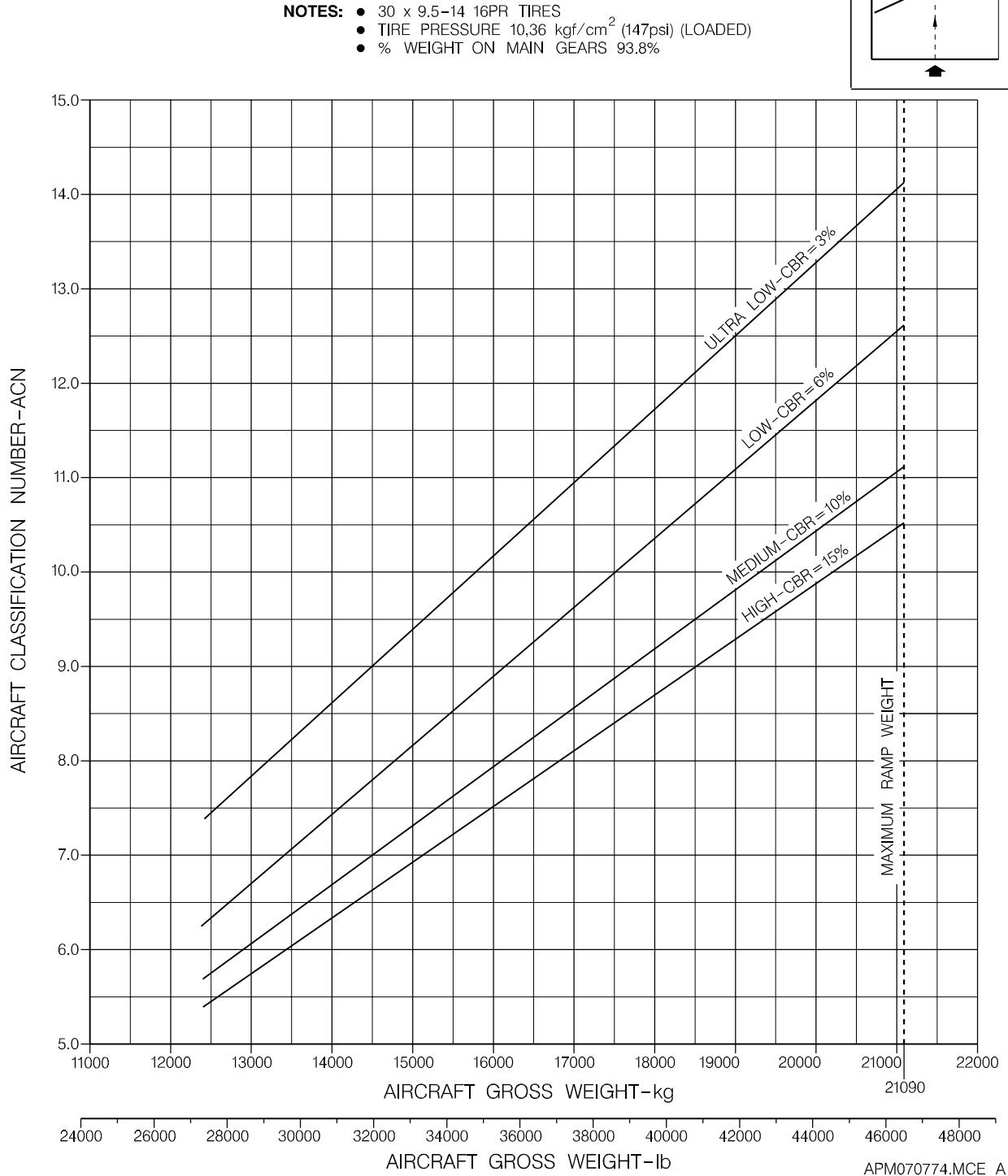
Figure 7.9.1 - Aircraft Classification Number Flexible Pavement
