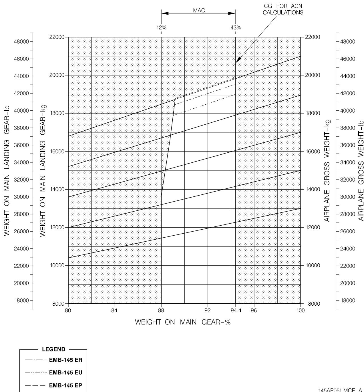
*Figure 7.4.1 - Landing Gear Loading on Pavement
