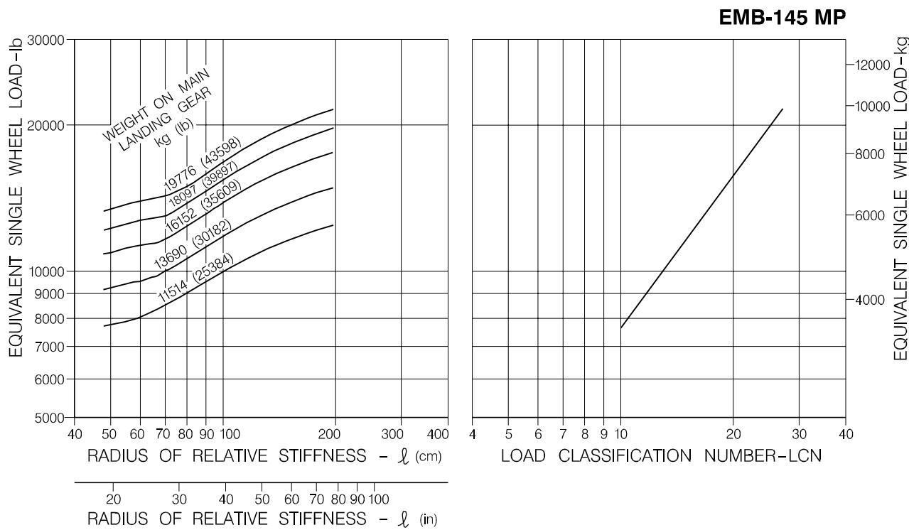
**NOTE:** EQUIVALENT SINGLE WHEEL LOADS ARE DERIVED BY METHODS SHOWN IN ICAO AERODROME MANUAL, PART 2, PAR. 4.1.3
