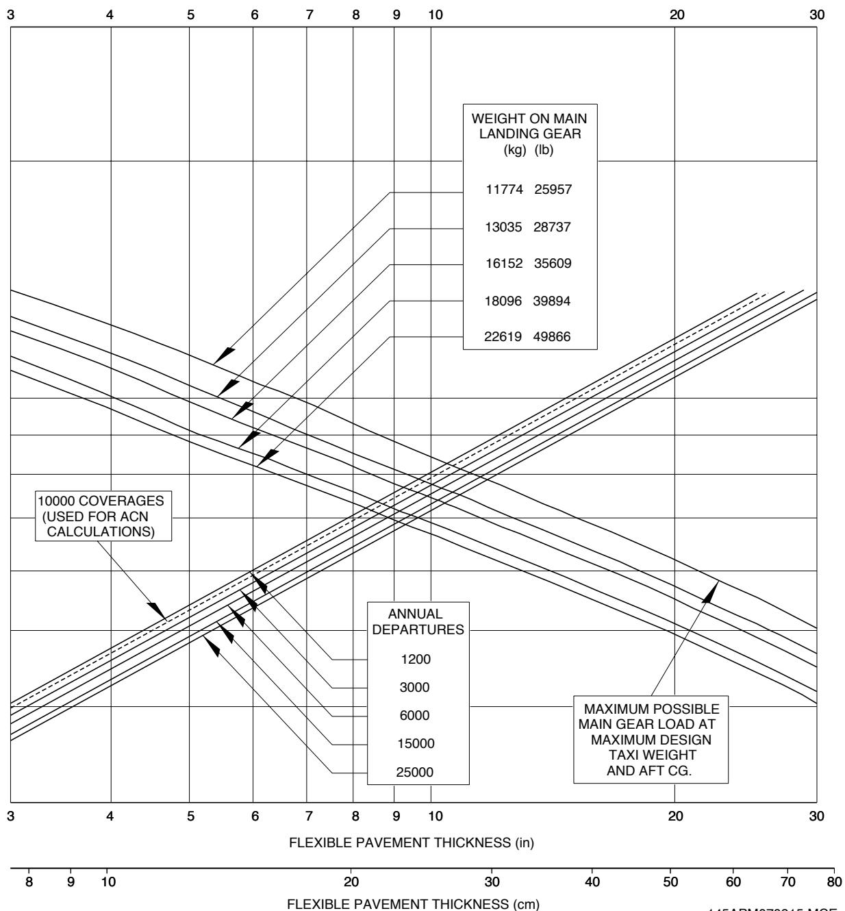
Figure 7.5.1 - Flexible Pavement Requirements - US Army Corps of Engineers Design Method
