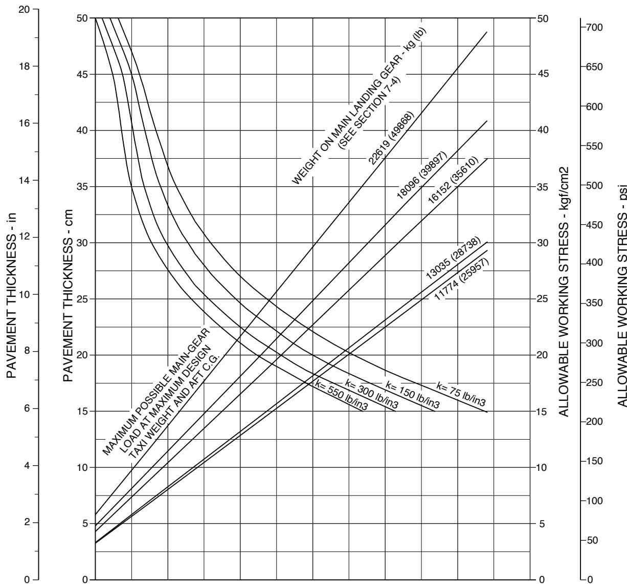
NOTE: THE VALUES OBTAINED BY USING THE MAXIMUM LOAD REFERENCE LINE AND ANY VALUE OF "K" ARE EXACT. FOR LOADS LESS THAN MAXIMUM, THE CURVES ARE EXACT FOR K=300 BUT DEVIATE SLIGHTLY FOR OTHER VALUES OF "K".
