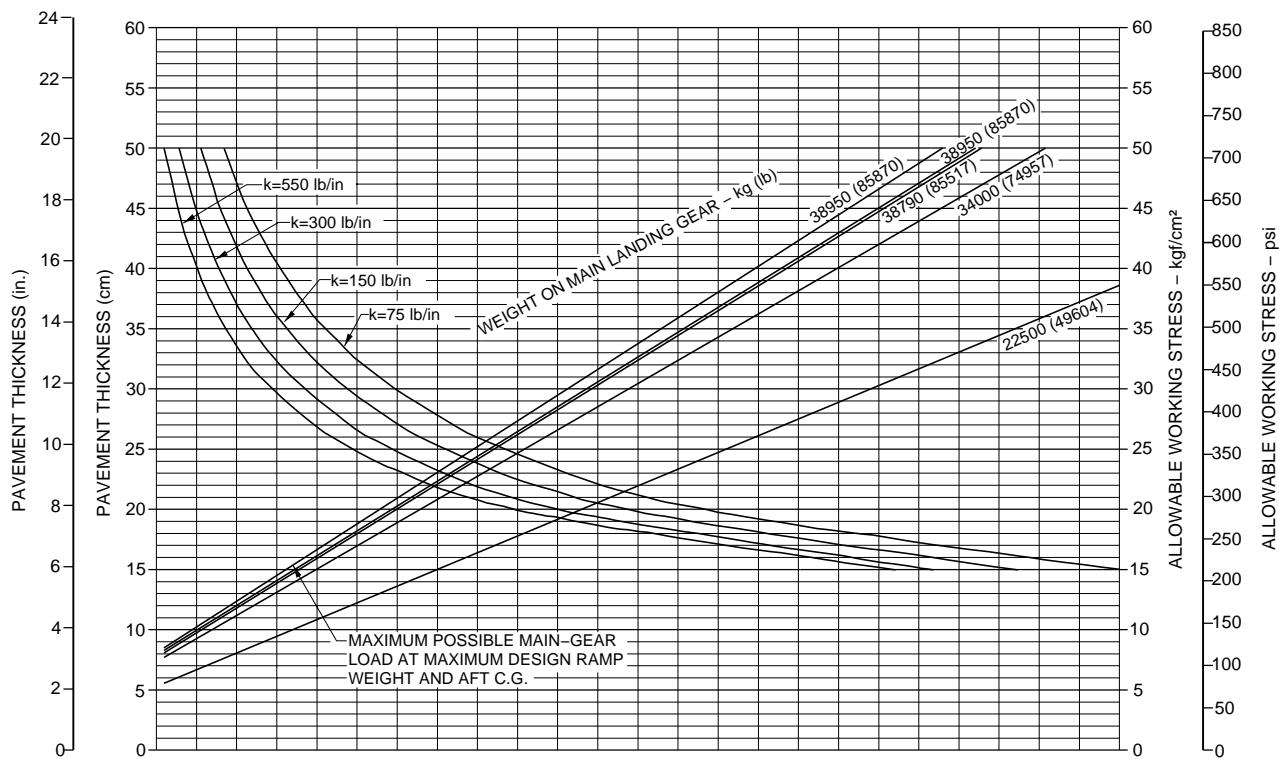
NOTE: THE VALUES OBTAINED BY USING THE MAXIMUM LOAD REFERENCE LINE AND ANY VALUE OF "K" ARE EXACT. FOR LOADS LESS THAN MAXIMUM, THE CURVES ARE EXACT FOR K=300 BUT DEVIATE SLIGHTLY FOR OTHER VALUES OF "K".
