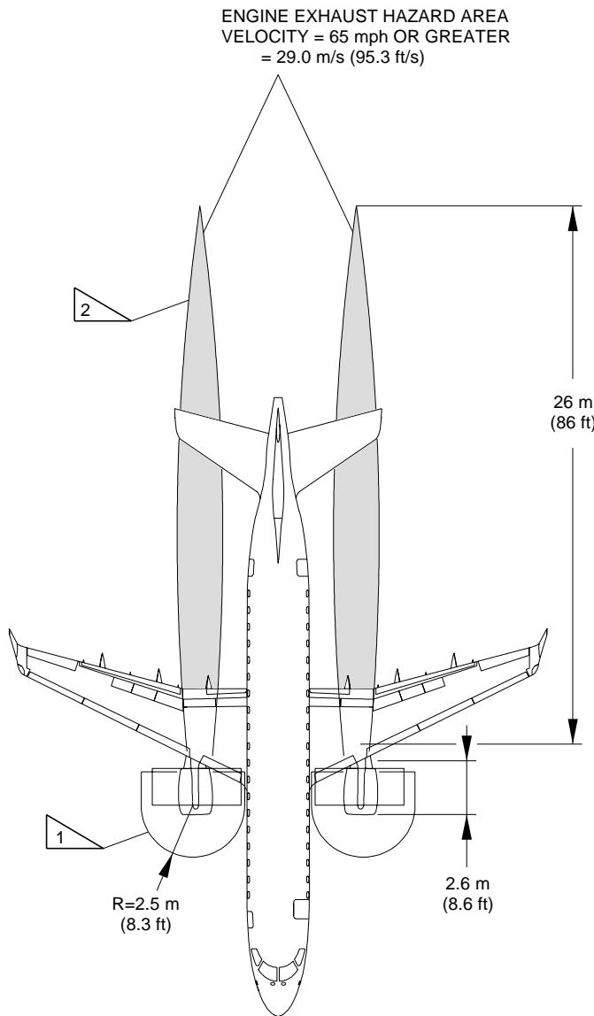
1 INLET HAZARD AREA – CONDITION: 20 kn HEADWIND/CROSSWIND/TAILWIND BASED ON 12.2 m/s (40 ft/s) CRITICAL VELOCITY WITH 0.9 m (3 ft) CONTINGENCY FACTOR.
