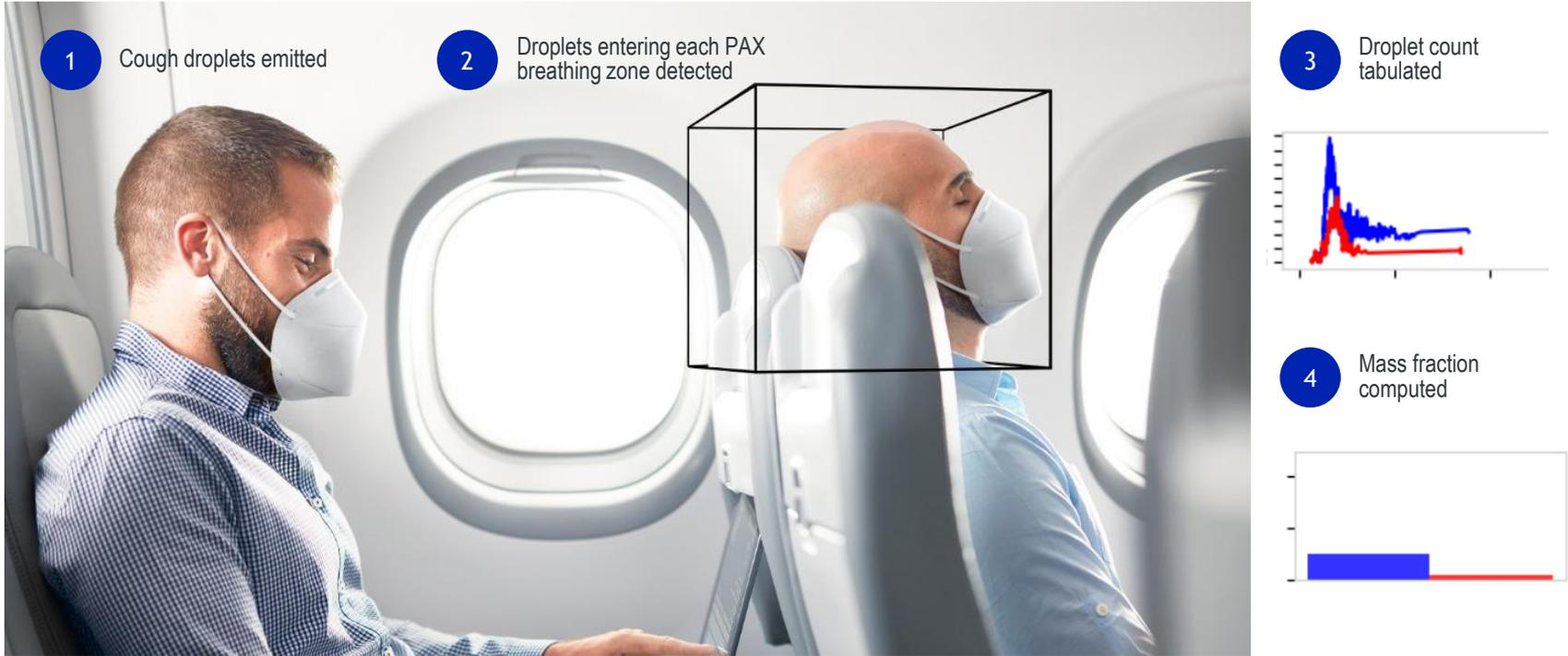
7-row CFD droplet dispersion model, 200  $\mu\text{g}$  in a cough distributed in 16 droplet diameters from 0.1  $\mu\text{m}$  - 200  $\mu\text{m}$
